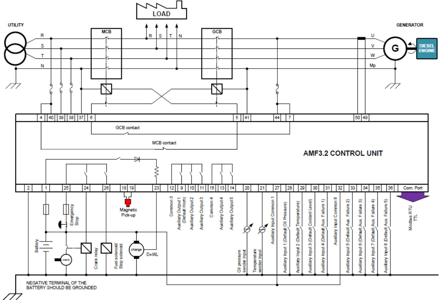
Typical connection diagram is shown and this is one of possible applications among many. The system is shown in 3 phase connection but can also be applied for single phase systems.
